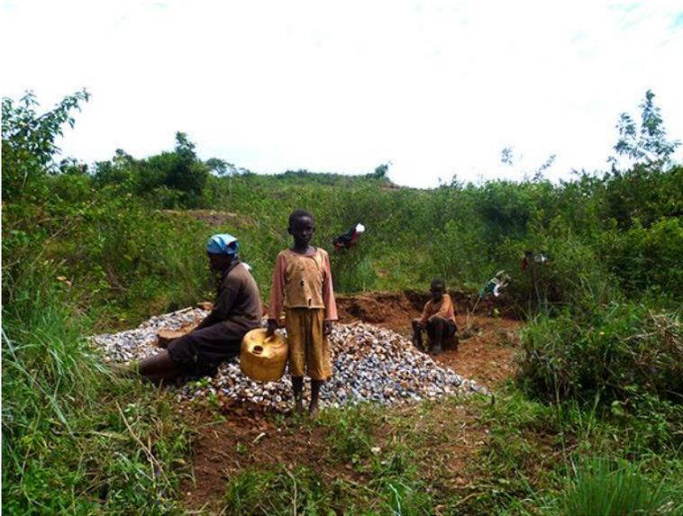
Hard core for the foundations is produced by manual labour in and around the village area. Individuals and families will work long hours to quarry a grade of stone suitable for our buildings. They are paid a local rate for their work.
